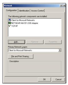
You must have an Ethernet adapter or an WG121, the TCP/IP protocol, and the Client for Microsoft Networks.
